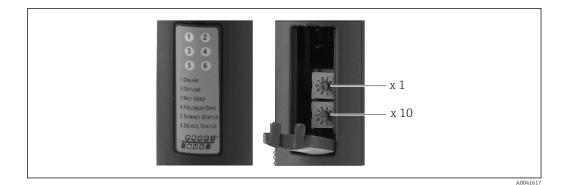
Using these rotary switches, a bus address in the range between 00 and 99 can be configured.  $\,$
