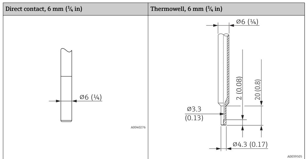
**i** It is possible to verify the mechanical loading capacity as a function of the installation and process conditions using the online TW Sizing Module for thermowells in the Endress+Hauser Applicator software → [30](#).
