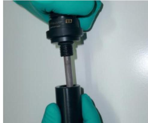
Figure 4+5: Disassembling of the measuring chamber
