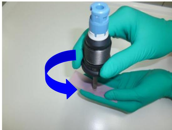
For polishing the cathode use the foils supplied by the maintenance kit. Wet the foil with a bit of water or electrolyte. Polish by rotating movement with the following sequence:
